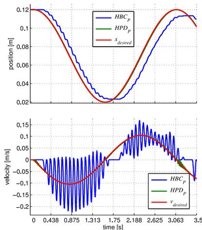
Fig. 13: Simulation of sinusoidal trajectory with P-controller
