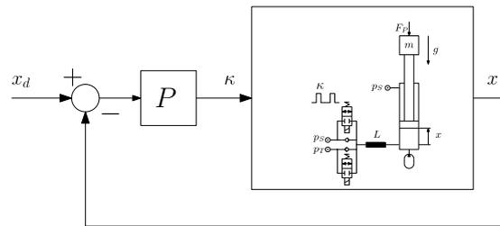
Fig. 12: Control scheme with P-controller
