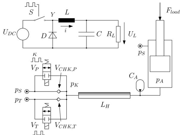
Fig. 1: Electric and hydraulic buck converter schematics
